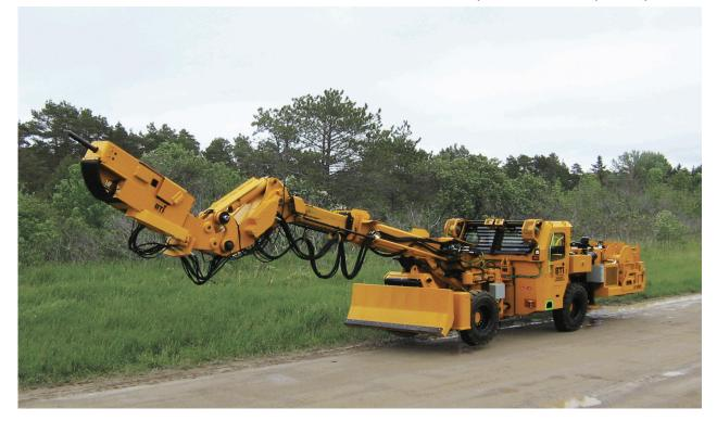
The hydraulic force-controlled breaker feed advancing along its longitudinal axis avoids jamming of the tool and provides controlled scaling of the mine ceiling.
