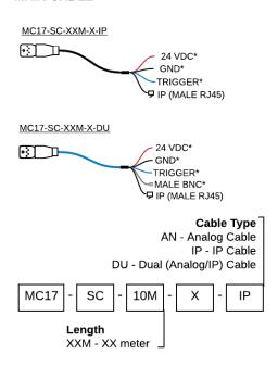
Main cable can be used in IP camera ToughCam-1000 installations. The IP cable includes a shielded Cat-5e cable for 10/100 Base-T signal transmission.
