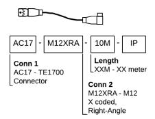
M12 adapter cables can be used in all IP camera TC10 installations. These cables take advantage of PoE input to reduce cabling complexity and cost.
